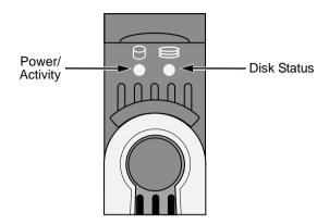
Figure 16. VTrak M500f/i/p drive carrier LEDs
